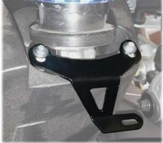
REMOVE THE ORIGINAL CHAIN COVER FROM THE MOTORBIKE AND THE TWO SCREWS FROM THE REAR SHOCK ABSORBER. USE THE TWO THICKNESS TO FIX THE BRACKET LIKE DESCRIBED IN THE PICTURE. ONCE FIXED THE BRACKET WE ADIVCE TO SEPARATE THE ABS PART FROM THE ALUMINIUM CHAIN COVER SO YOU CAN FIX ON THE MOTORBIKE.
